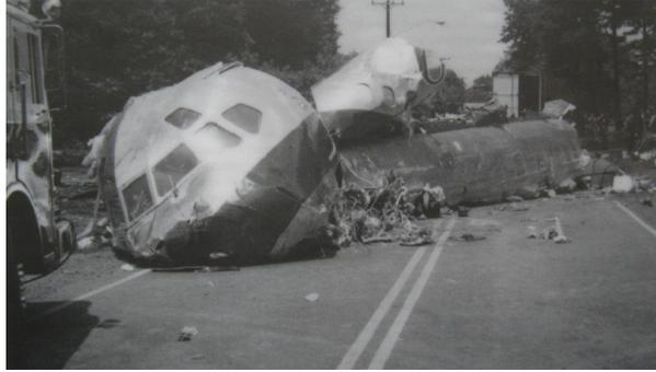
Figure 1: Remnants of the aircraft N954VJ involved in USAir Flight 1016 [141]. The plane crash was attributed to the lack of warnings about wind shear from the air flight controller on duty who, due to mistrust in the wind shear alert system, reported only one out of three alerts generated by the system.
